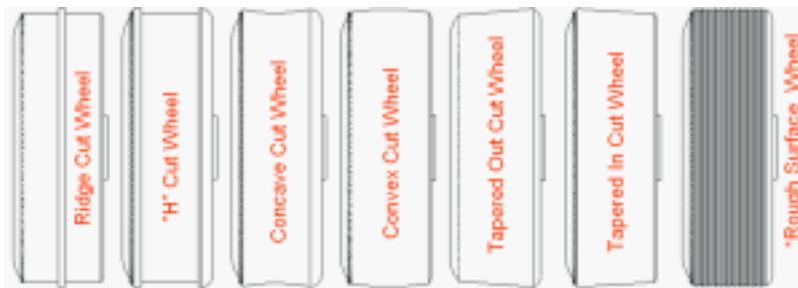
Examples of Illegal Wheel Tread Modifications
